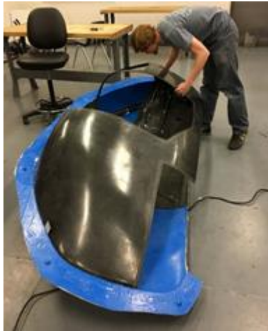
Figure 32: Fairing Removal from Mold
